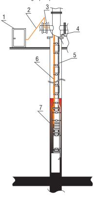
1 – dosing unit: 2 – onshore pipeline: 3 – input device through the lateral branch of the fountain fittings; 4 – input device through the cable input of the fountain fittings; 5 – power cable of the ESP system; 6 – downhole capillary tube; 7 – spray valve
