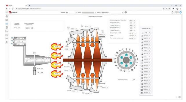
Mnemonic diagram of a gas turbine in the interface of the PRANA hardware-software package
