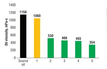
FIGURE 8. Example of modeling results of the use of complex technology for treating the formation zone of a vertical well with solvent and steam at a high-viscosity oil facility (oil saturated thickness 14 m, oil viscosity under formation conditions 400 mPa·s, pre-injection of aromatic solvent reagent bank)
